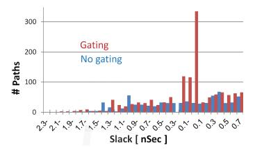
Fig. 5. Negative slack distribution in the 3-D graphics accelerator [9], [25], for 200-MHz clock cycle. The introduction of clock gating resulted in a few additional delay paths with negative slacks.
