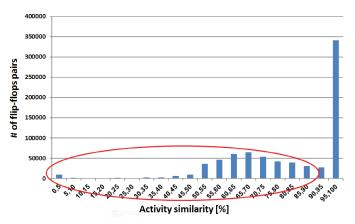
Fig. 3. Activity similarity of FFs in a DSP core (see Fig. 1). FFs are paired only if they share same pre-enabled clock signal. Undesirable pairs are encircled.
