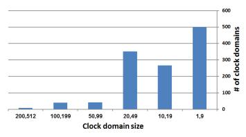
Fig. 4. Distribution of the number of FFs sharing a common pre-enabled clock signal of a DSP core (see Fig. 1).
