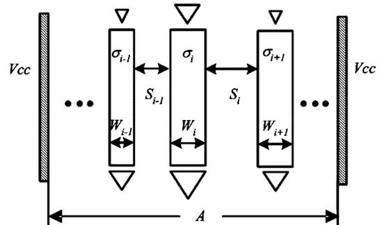
Fig. 1. Structure of the bus:  $n$  parallel signal wires share a fixed total width  $A$  between two shield wires.
