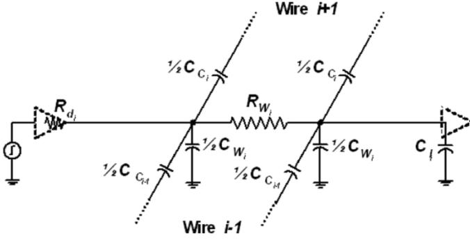
Fig. 2. Equivalent circuit for calculating the  $i$ th signal delay.
