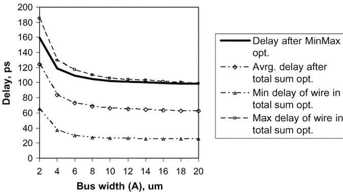
Fig. 10. Optimal solution parameters  $\Delta'$ ,  $\Delta^{\sim}$ ,  $\Delta^*$ ,  $\Delta''$  (see Fig. 4) versus bus width constraint A, for the circuit of Example 4.
