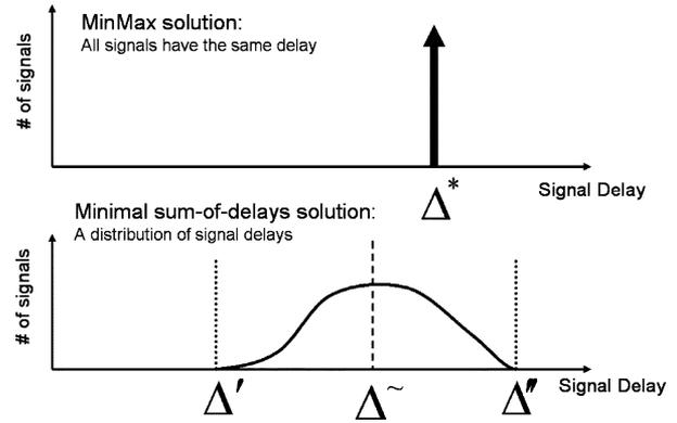
Fig. 4. Distributions of signal delays in MinMax solution (top) compared with minimal sum-of-delays solution (bottom).
