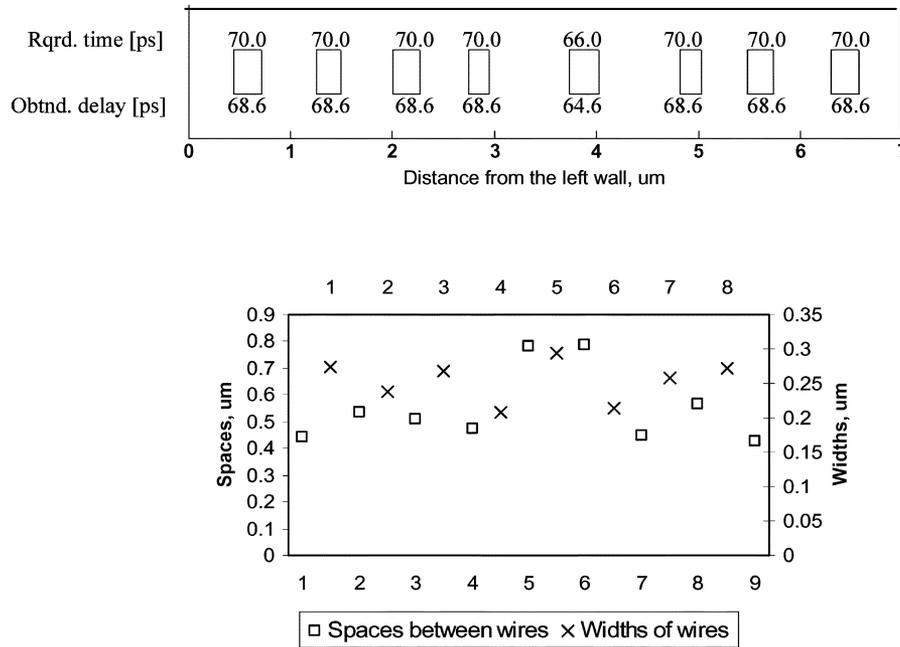
Fig. 7. (Top): cross section of the bus after MinMax slack optimization. (Bottom): width and spaces shown as graphs versus wire position in the bus.
