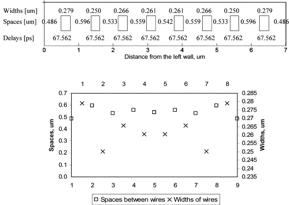
Fig. 5. (Top): cross section of the bus after MinMax delay optimization, annotated with values of wire widths and spaces. (Bottom): width and spaces shown as graphs versus wire position in the bus.
