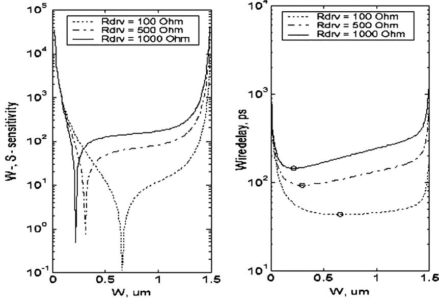
Fig. 3. Delay sensitivity to width and space for a single wire.
