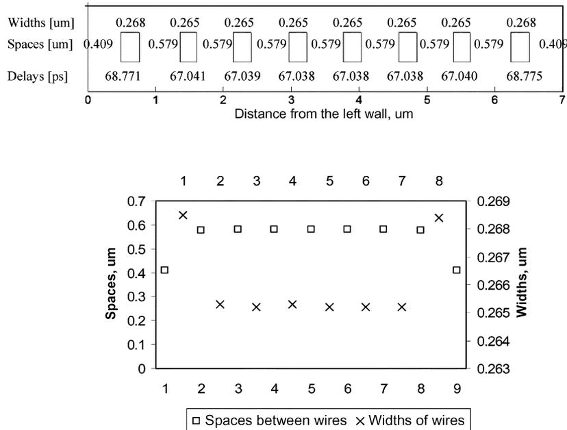
Fig. 6. (Top): cross section of the bus after sum-of-delays optimization, annotated with values of wire widths and spaces. (Bottom): width and spaces shown as graphs versus wire position in the bus.
