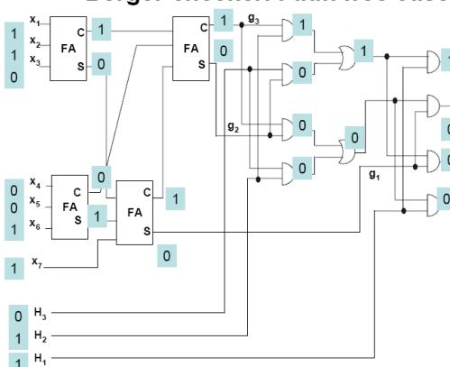
Berger checker (fault in a functional circuit)
