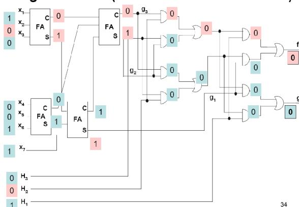
Berger checker (stuck-at-1 fault in the checker)
