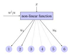
**Fig. 1**. The dropout soft-max layer, where the edges that do not belong to the cluster of the trained label are dropped. In this illustration the correct class is 1 and  $c(1) = \{1, 2, 6\}$ .
