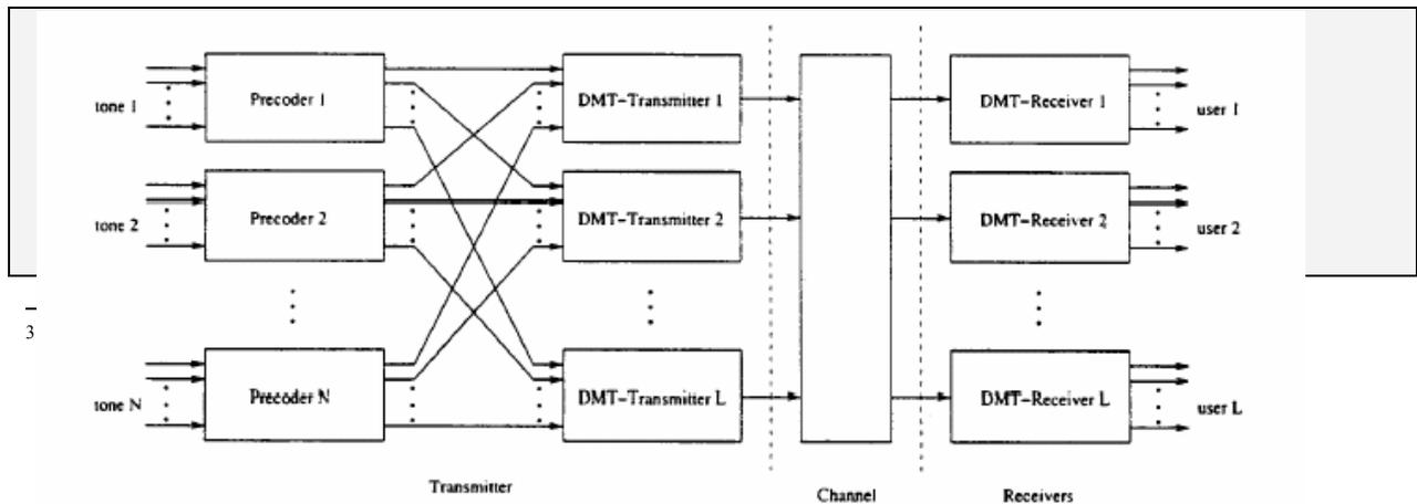
Figure 3 – linear precoding illustration.
