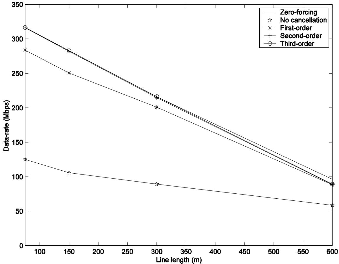
Figure 4 – Results of differential excitation and linear precoder (per line).
