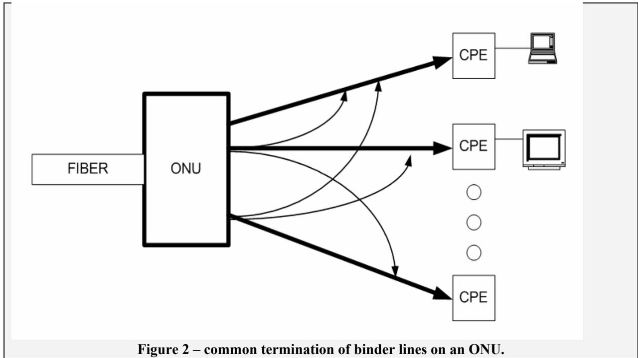
Figure 2 – common termination of binder lines on an ONU.
