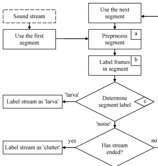
**Fig. 4 – Flow diagram describing the detection algorithm used to analyze sound files.**
