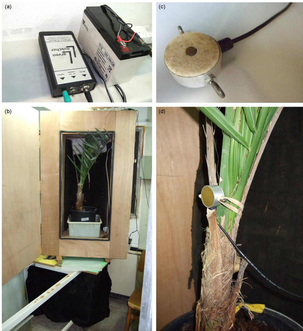
**Fig. 3 – (a) Amplifier and a 12 V, 7 Ah battery. (b) An offshoot inside the sound-isolated box. (c) Piezoelectric microphone. (d) Microphone attached to offshoot's stem with a rubber band.**
