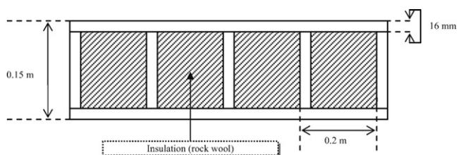
**Fig. 1 – Sound-isolated box wall section. Each wall was 0.15 m thick, constructed from two layers of 16-mm plywood, braced with orthogonal braces.**
